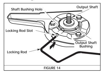
2. Hold the locking rod in place by grasping it next to the boom of the unit. See Figure 15.
